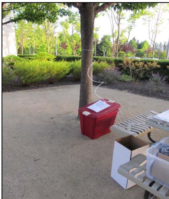
Outdoor air sample placed near the building perimeter.
