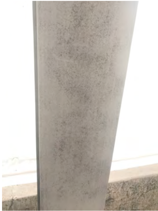
Photograph 8 – Structural steel after removal of paint/coatings with media blast system. Light areas are referred to as ‘white metal.’ Darker areas are residual mill scale.
