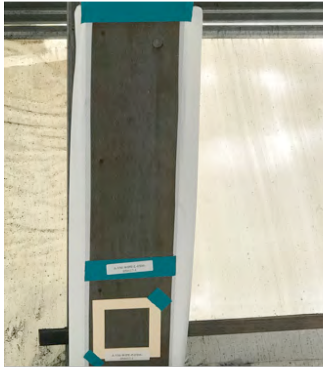
Photograph 15 – Structural steel after removal of paint/coatings at time of verification sampling.
