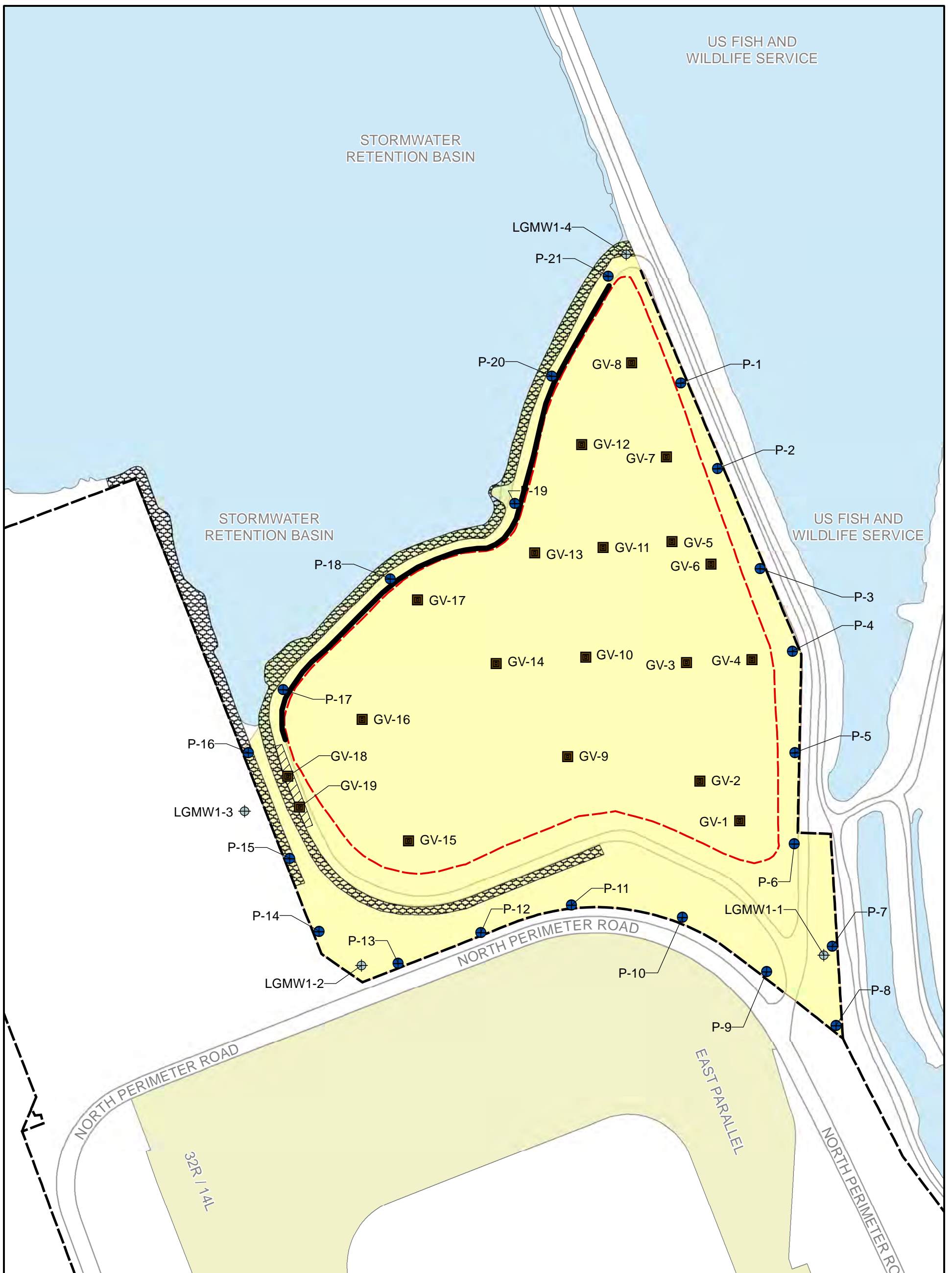
Ames Research Center Moffett Field, CA 94035 FIGURE 9 SITE 1 LANDFILL METHANE MONITORING LOCATIONS
